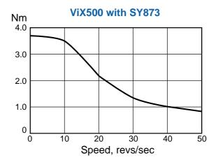
Figure 3-2. Stepper Drive Torque/Speed Data
